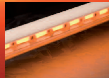
Processing of silicon with a QRC® heater
