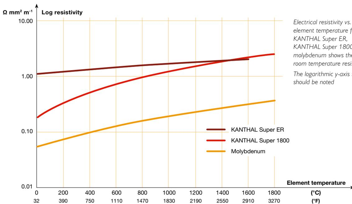
Electrical resistivity vs. element temperature for KANTHAL Super ER, KANTHAL Super 1800 and molybdenum shows the high room temperature resistivity. The logarithmic y-axis scale should be noted.
