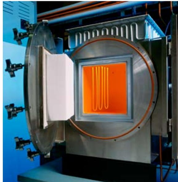
is often used. Operation in air or oxidizing atmospheres, however, is not possible due to the detrimental oxidation of molybdenum to MoO<sub>3</sub>.
