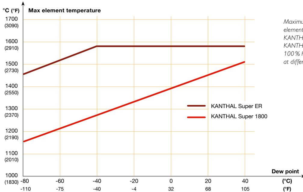
Maximum recommended element temperature for KANTHAL Super ER and KANTHAL Super 1800/1900 in 100% hydrogen (H<sub>2</sub>) atmosphere at different dew points
