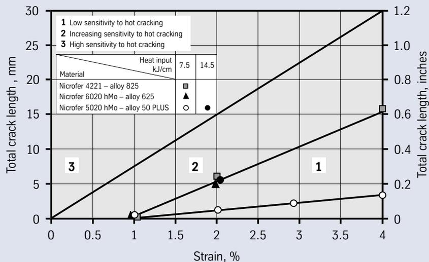
Fig. 4 - Hot cracking behaviour of Nicrofer 5020 hMo in comparison with Nicrofer 6020 hMo and Nicrofer 4221 in the Modified Varestraint Test (MVT).
