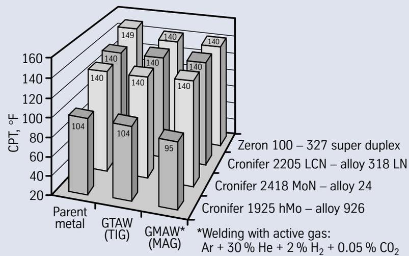
Fig. 3 - Critical pitting temperatures of weld joints of 6-Mo, high nitrogen austenitic, duplex and super duplex stainless steels with Nicrofer S 5020 – FM 50 filler metal in "green death" test solution.
