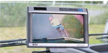
The camera delivers a true-sided image. The picture on the monitor is crystal-clear, bright and high in contrast.
