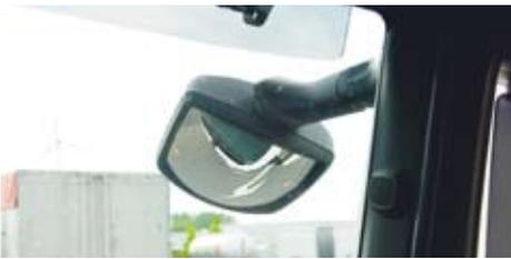
The mirror produces a reversed and distorted image. The driver's line of vision is outside the wiper area.
