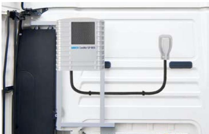
Quickly done: installation and connection of the condenser unit. The condenser fastening frame uses the vehicle's existing fastening points.
