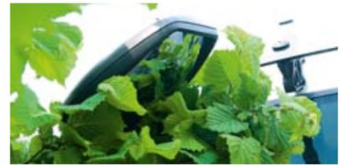
The front mirror protrudes over the sun visor: risk of damage in the wash bay, by tree branches, or when manoeuvring.
