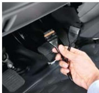
Connection to the accelerator via T-plug
