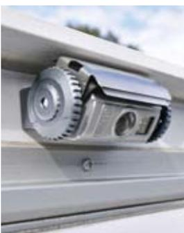
Automatic, motor-operated shutter to prevent soiling of the camera lens
