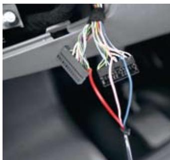
Signal tapped with just three vehicle-specific plug-in connectors
