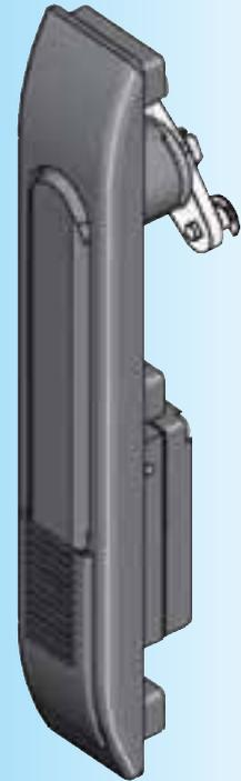
Swinghandle with push button (2100-U57), handle zinc die black powder coated, shaft zinc die zinc pl., escutcheon polyamide GF black, fixing material m.s. zinc pl., fixing bridges polyamide GF black, with seal
