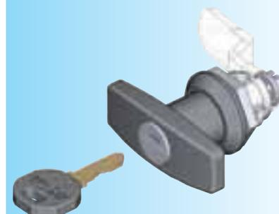
Handle polyamide GF black, housing zinc die black p.c., cylinder zinc die with stainless steel cap and shutter, nut, earthnut and fixing material m.s. zinc plated.
