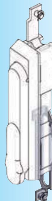
The use of this connector in conjunction with rod controls (3YA-160) version B gives a smaller width. In the case of installation of the long escutcheons or swinghandles with rear cap mounted at the door centre the length of the upper and lower rod will be the same.
