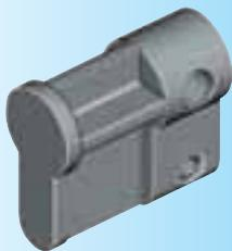
EMKA profile half cylinder with round cylinder zinc die with stainless steel cap and shutter with one key silver steel with grip polyamide GF black, turn 360°.
