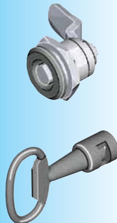
**Housing zinc die or PA and insert zinc die zinc plated, nut and earthnut m.s. zinc plated**
