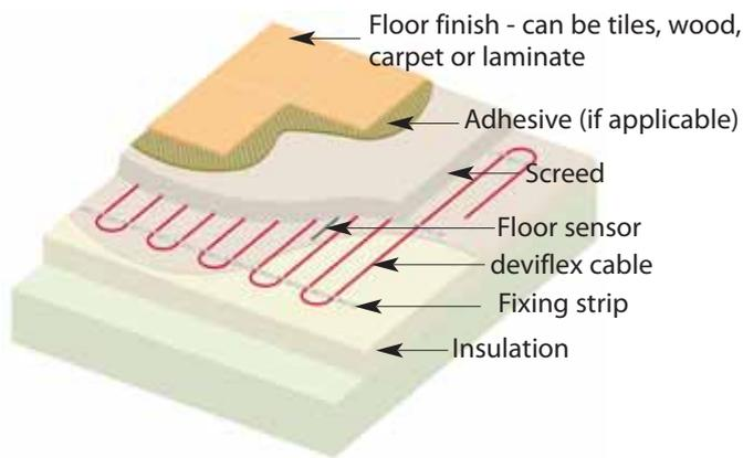
Here the insulation is laid on top of the concrete slab, followed by the heating cable. The cable is covered with a minimum of 65mm\* sand and cement screed. The chosen floor covering is then laid; this can be tiles, wood, laminate, carpet or vinyl.
