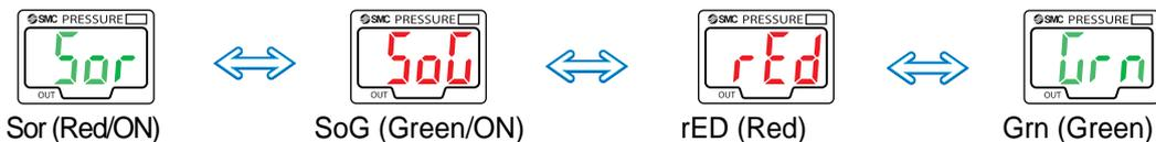
Press the **[SET]** button to set the desired display color and to move on to setting a desired operation mode. If the mode is set to analog output, press the **[Δ]** or **[▽]** button, to select a desired display color from "Grn (Green) ↔ rED (Red)", then press the **[SET]** button. Setting of a desired measurement mode will become available.
