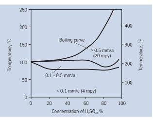
Fig. 2 – Isocorrosion diagram of Nicrofer 5716 hMoW-alloy C-276 in lightly aerated, technical grade sulphuric acid based on immersion test results over at least 120 h.
