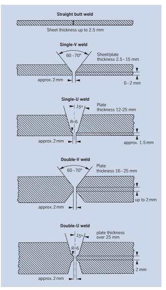
Fig. 3 – Edge preparation for welding of nickel-base alloys.
