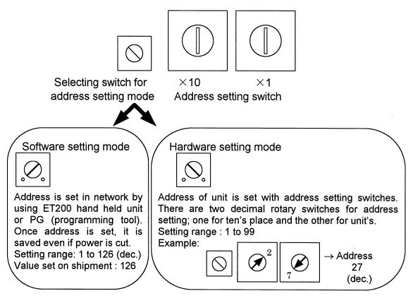
\*When software setting mode is selected, address setting switches are not effectual. Moreover, software setting mode and hardware setting mode differ in ID numbers of units. (See "12. Configuration" for details.)
