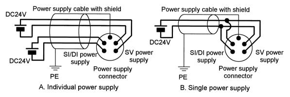
Power for SI/DI units is also distributed to sensor connected with DI unit. Select sensor concerning voltage drop inside the unit. It may reach approximately 2V at the maximum. If sensor requires 24V, it is necessary to lower power supply voltage for SI/DI unit slightly or secure power supply for sensor separately without going through SI unit so that sensor input voltage can be 24V with actual loading (allowable voltage of SI/DI unit power supply: 19.2V to 28.8V).
