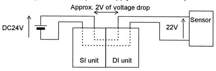
Select power supply cable sufficient for power consumption and number of stations of solenoid valves, and current consumption of SI unit and sensor.
