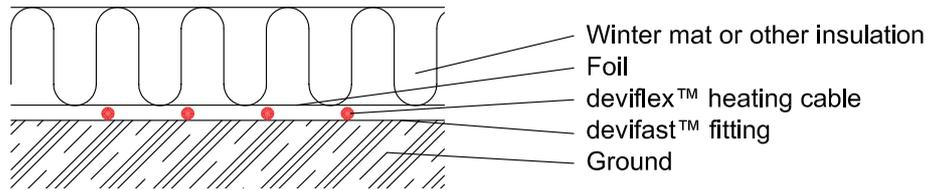
The day before the hole is to be dug, 44 m of deviflex™ DTIP-18 heating cable is laid with a total output of 790 W. The cable is laid on devifast™ fitting bands with a C-C distance of 5 cm, providing an output of 360 W/m<sup>2</sup>.
