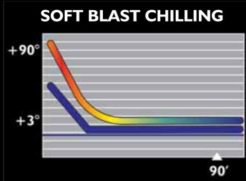
**SOFT Blast Chilling Cycle** is recommended for delicate, light, thin or small portions of food..
