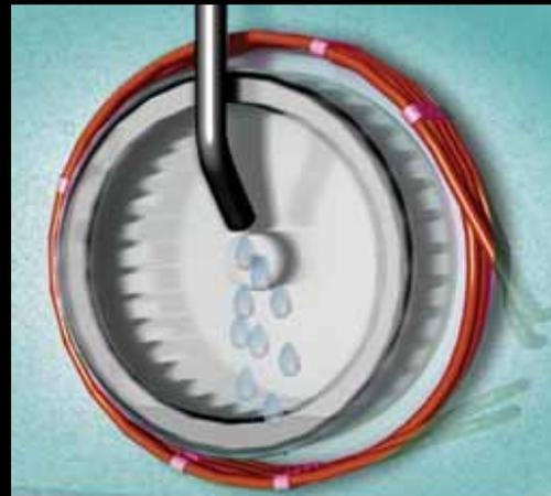
With this revolutionary system, that replaces the traditional boiler, the water entering the chamber is nebulized by fans and vaporized on the heating element. The steam is produced immediately and starting from the temperature of 70°C.
