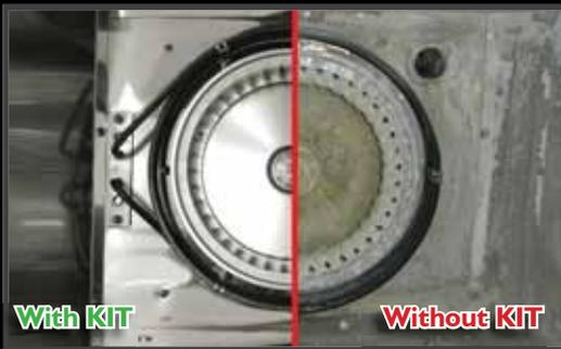
It is well-known that the presence of lime scale, minerals and other water impurities produce scale on the heating elements, ferrous residuals in the cavity, scale on the fans, with consequent loss of balance and problems for the motors. All this will result in a reduced life of the oven.
