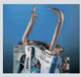
Efficient technology mix: servo-pneumatic welding tong with roughly 25 % less compressed air consumption than conventional welding tongs
