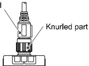
1. Insert the lead wire attached with a connector into the key groove.
