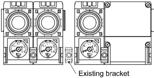
1. Loosen the screws and dismount two brackets one each front and back surface.
