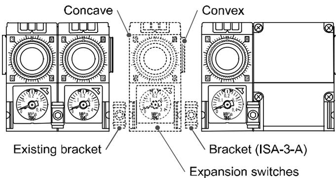
1. Set the expansion packing (ISA-7-B) in the concave of the SUP port for expansion switches.
