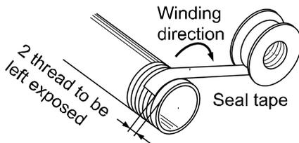
When using tape sealant, leave a couple of screw threads unwrapped with tape sealant.
