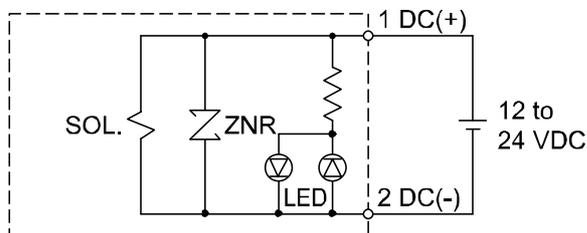
See the catalog and operation manual of SMC VCA series for the wiring method of circuit and wiring for 2-port solenoid valve.
