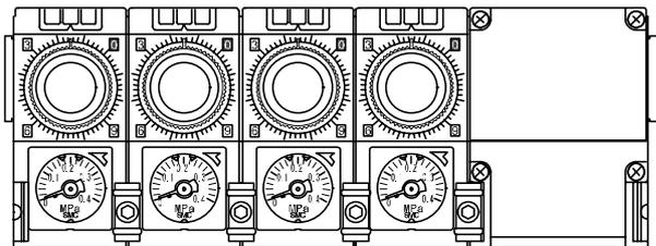
1. Tightening the fasteners by specified torque 1.2 Nm.
