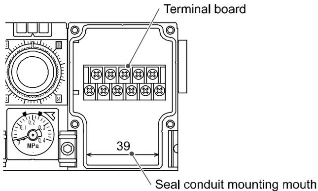
1. Mount the seal conduit on the terminal board box. See the catalog and operation manual of the seal conduit manufacturer for the method to mount the seal conduit.
