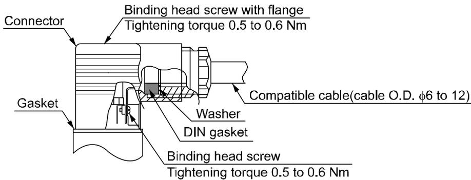
\*: Use after remove inner of DIN gasket in case of cable O.D. is  $\phi 9$  to 12.
