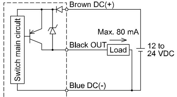
•Circuit and wiring for 2-port solenoid valve
