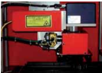
Integrated vision system (mark verification)
