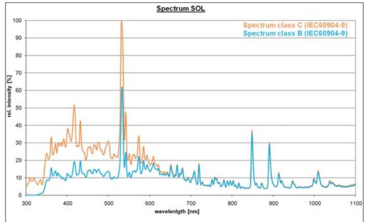
The irradiation of the SOL units generates a class C spectrum according to IEC60904-9. Class B can be achieved by using of appropriate filters.
