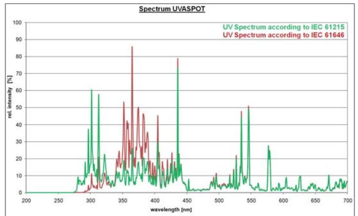
For UV preconditioning tests the spectrum of our UVASPOT units can be adopted to the relevant requirements of IEC61215 and IEC61646 by the usage of different filters.
