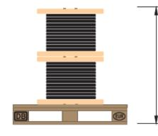
Maximum loading height, incl. pa**ll**et 1190 mm
