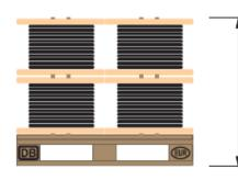
Maximum loading height, incl. pa**ll**et 1190 mm
