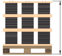
Maximum loading height, incl. pallet 1190 mm
