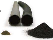
Comparison of APMT tube versus Fe-35Ni-25Cr after 2300 hours at 1100°C (2012°F). The FeNiCr tube is severely contaminated with oxide flakes.
