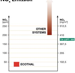
Typical  $NO_x$  emissions of different burner systems. ECOTHAL SER-burner is far below 350 mg/m<sup>3</sup>.
