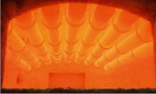
Kanthal TUBOTHAL is an ideal electric element used in combination with PM tubes because of its great advantages, such as – very high power – long life – low weight – easy to design to existing power controls and supply. Combined with APM tubes, a “maintenance free system” is obtained with high reliability and with no need to remove elements, clean or rotate tubes, if correctly designed.
