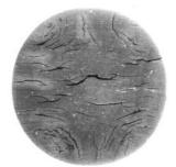
This phenomena is known as Explosive Decompression (ED). Cracks and blisters may be evident on the surface of the seal, they may be internal, or they may only be detected by magnification.
