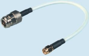
Adapter cable (N female/RP-SMA-Plug), attenuation 0.5 dB at 2.4GHz, 1dB at 5GHz
