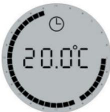
In connection with the built-in Timer, the thermostat can be programmed to lower the temperature (LO), e.g. during the night.
