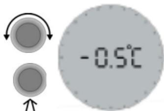
Due to different floor constructions it is possible to choose a maximum floor temperature (**Mt**) in the floor which cannot be exceeded.
