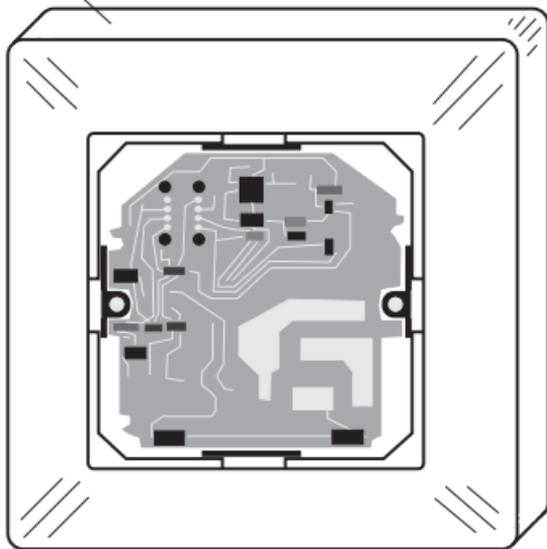
Remove the two screws, one in each side, and gently pull off the display module.
