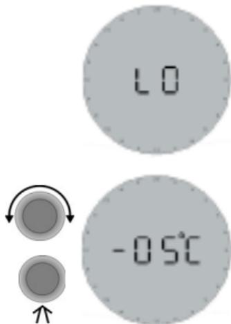
Offset (OFFS) can be used to adjust a variation between the thermostat and a thermometer in the room, if any. If the thermometer shows e.g.  $1^{\circ}\text{C}$  more than the thermostat, it is possible to adjust the offset with  $+1^{\circ}\text{C}$ . The range is  $-5.5^{\circ}\text{C}$  to  $+5.5^{\circ}\text{C}$ .
