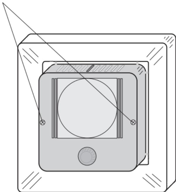
Reassemble the thermostat by first placing the frame, then mount the display module and finally press the front cover into place.
