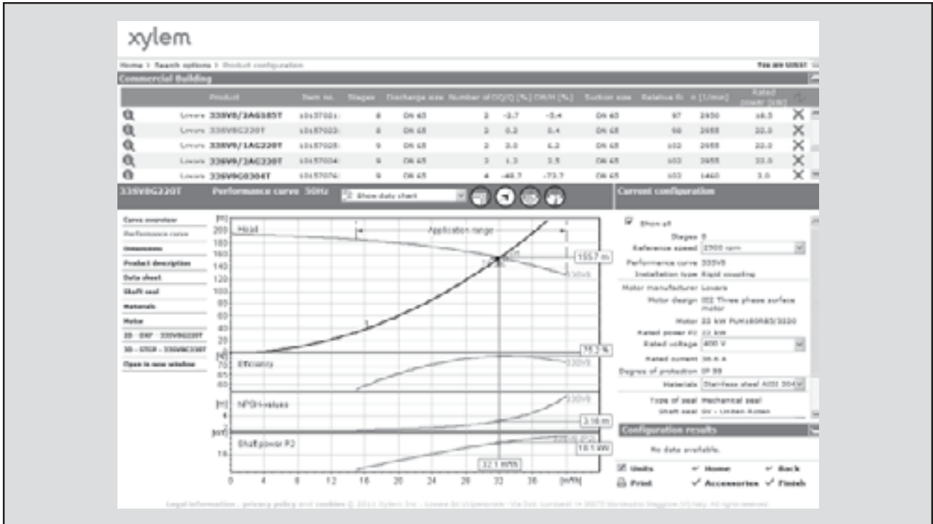
The detailed output makes it easy to select the optimal pump from the given alternatives.
