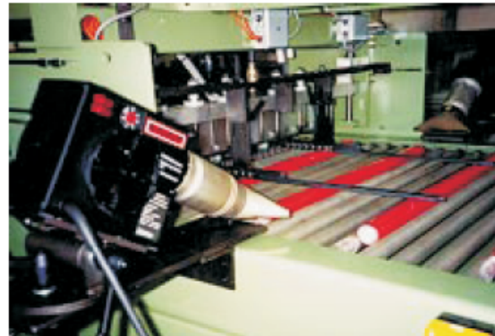
A Hotwind S used for side shrinking of wrapped decorative film.
