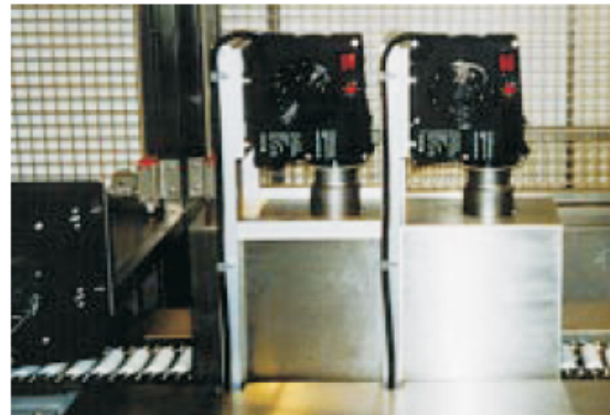
Hot air equipment with two Hotwind S and a Heater 700 used to shrink PE covers on batteries.
