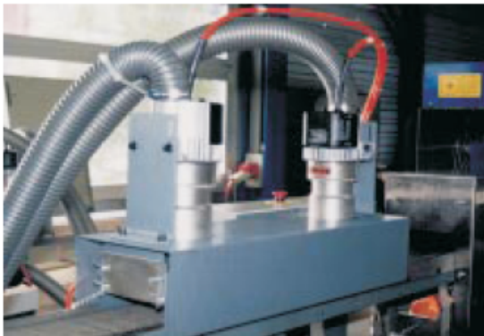
Heating of a shrinking tunnel with two Heaters 10000 S. The Silence medium pressure blower supplies the air.
