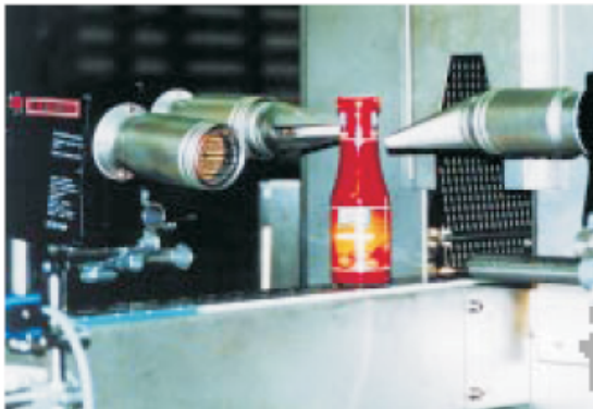
Three Hotwind S used on to shrink caps on to bottles. A frequent application for fruit-juice and wine bottles.
