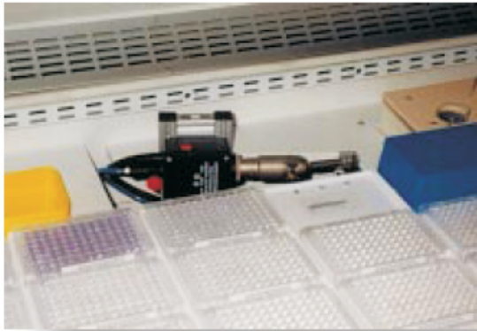
A Heater 700 hot air tool and Robust blower used to sterilise test needles.
