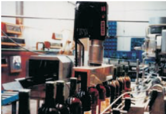
Hotwind S with push-fit shell reflector, installed in a bottle filling machine used for shrinking caps.
