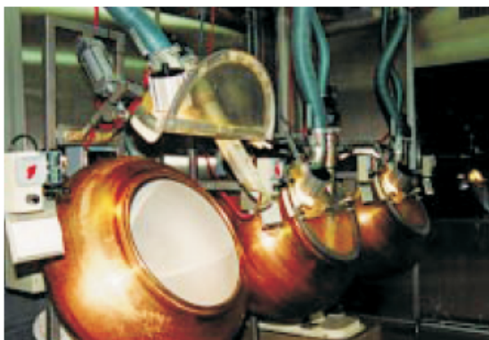
Drying and smoothing pills, tablets, sweets and their coatings with several Heaters 5000 and ASO blower. The KSR is used for accurate temperature control.
