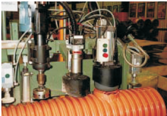
A Heater 5000 and Robust blower used to warm up PVC tubing. Subsequent shaping to form branches presents no difficulties.
