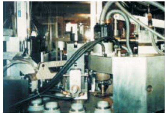
Welding plastic tubes with a Heater 3000 and Robust blower. The ends of tubes for toothpaste, ointment and adhesives are welded with hot air after being filled.
