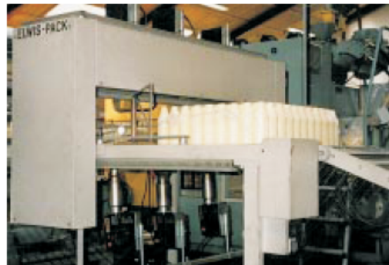
Hot air installations in a shrink tunnel for shrinking and welding film on bulky goods.
