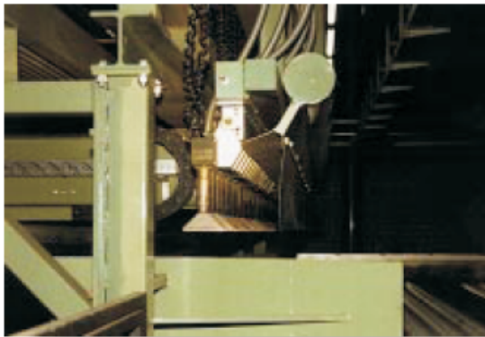
40 Heaters 3000 and 24 Heaters 700 burn marking lines (transverse and longitudinal) in sheets of insulation without using paint.
