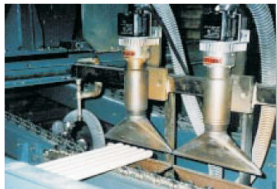
A Heater 5000 and ASO blower used to heat the ends of fluorescent tubes. This removes the coating before gluing.
