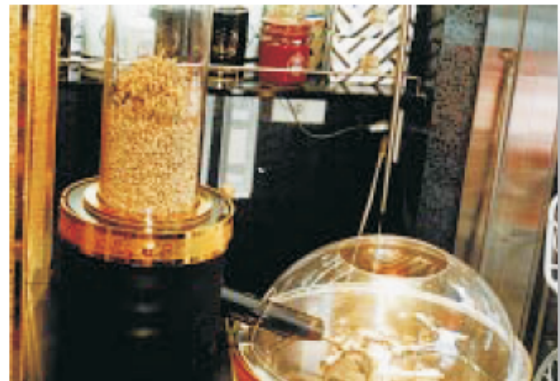
A Heater 5000 and Robust blower provide hot air for a coffee roasting machine. The temperature of the hot air and the roasting time can be set according to the customer's requirements via computer.
