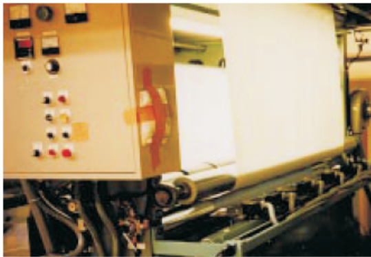
Six Heater 3000 fitted with 70 mm wide slot nozzles built into a plastic welding machine used to weld polyester fleece to EVA foils.
