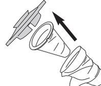
Twist and lift off lid; separate 2 filters.
