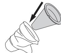
Replace inner filter into filter cover.
