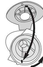
Align lid notch to filter rib and twist to lock.
