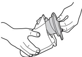
Reposition filter assembly inside dust cup.
