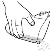
Remove filter assembly and empty debris.
