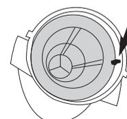
Align notch to rib and push inner filter down.
