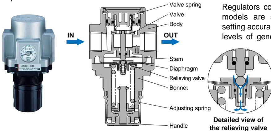
Regulators come in general-purpose and precision models are selectively used according to their setting accuracy. In most cases, the setting accuracy levels of general-purpose and precision regulators are approximately  $\pm 0.05$  MPa and  $\pm 0.01$  MPa, respectively. In general industrial machinery, general-purpose regulators are commonly used, while precision regulators are used only when high pressure accuracy levels are required.
