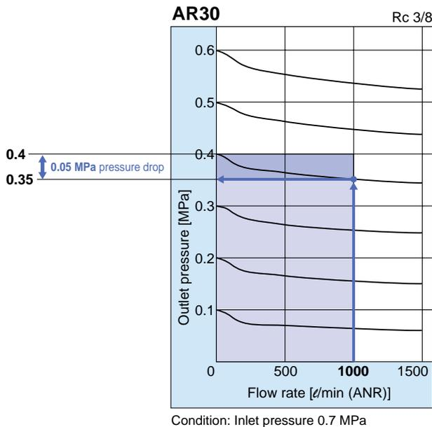
**Example: How to read the AR30's flow characteristics**
